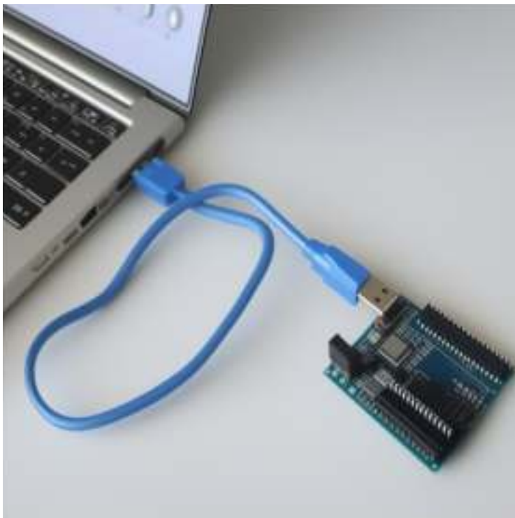
this is how to connect the microcontroller to a laptop
